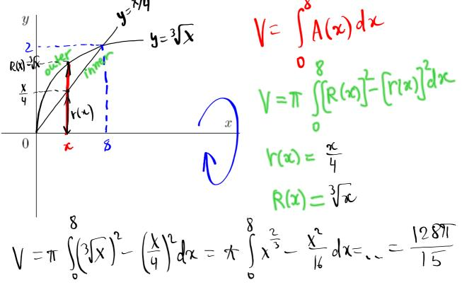
$$V = \pi \int_{0}^{8} (3\sqrt{x})^{2} - (\frac{x}{4})^{2} dx = \pi \int_{0}^{8} x^{\frac{2}{3}} - \frac{x^{2}}{16} dx = \frac{12871}{15}$$
