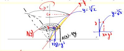
$$V = \int_{0}^{c} A(y) dy = \pi \int_{0}^{c} (R(y))^{2} - [r(y)]^{2} dy$$
