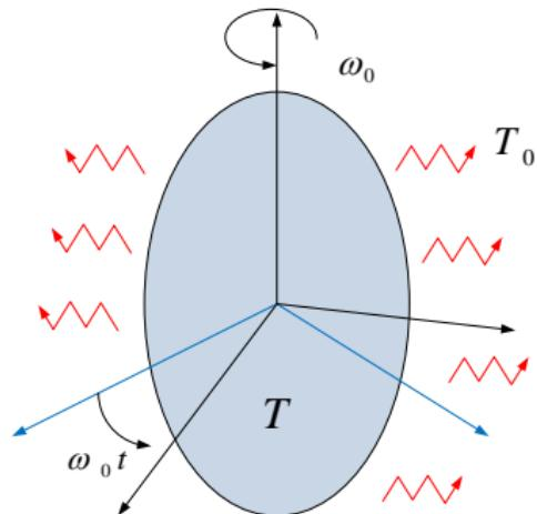
$$\begin{aligned}\rho' &= \rho, & \varphi' &= \varphi - \omega_0 t, & z' &= z, & t' &= t, \\ \partial_{\rho'} &= \partial_\rho, & \partial_{\varphi'} &= \partial_\varphi, & \partial_{z'} &= \partial_z, & \partial_{t'} &= \partial_t + \omega_0 \partial_\varphi,\end{aligned}$$
