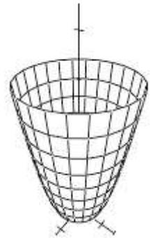
The cross section at height  $y$  is a circle of radius  $x = y^{1/4}$  and hence area  $A = \pi x^2 = \pi y^{1/2}$ . A slice of thickness  $dy$  has volume  $dV = A dy = \pi y^{1/2} dy$  and mass  $dm = \rho dV = \rho \pi y^{1/2} dy$ . This slice must be lifted a distance  $h = 30 - y$ .
