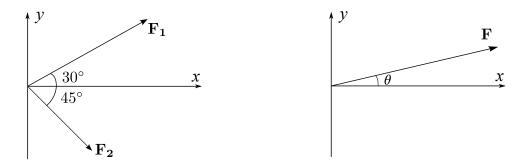
$$\mathbf{F_1} = |\mathbf{F_1}| \langle \cos 30^\circ, \sin 30^\circ \rangle = 34 \langle \cos 30^\circ, \sin 30^\circ \rangle = 34 \left\langle \frac{\sqrt{3}}{2}, \frac{1}{2} \right\rangle = \langle 17\sqrt{3}, 17\rangle$$
