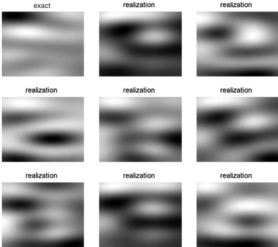
Fig. 6. Permeability realizations after each update. Random walk sampler with \sigma = 0.01 is used
