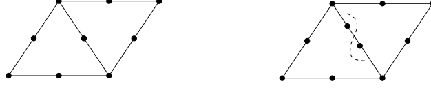
Fig. 1.19. Compatible (left) and incompatible (right) position of nodes at an interface for a geometrically conforming mesh.
