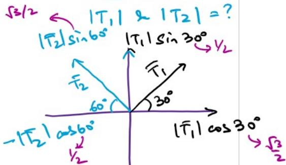
$$x: |\bar{T}_1| \frac{\sqrt{3}}{2} = |\bar{T}_2| \frac{1}{2} \Rightarrow |\bar{T}_2| = |\bar{T}_1| \frac{(\frac{\sqrt{3}}{2})}{(\frac{1}{2})} = \frac{|\bar{T}_1| \sqrt{3}}{2}$$
