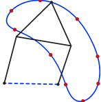
A four bar mechanism is a plane quadrilateral with a triangle mounted opposite a fixed side. The six 'bars' have fixed lengths, but rotate freely at their joints. The apex of the triangle traces out the *workspace curve*.
