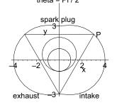
From  $\theta = \pi/2$  to  $\theta = 2\pi$ , the fuel expands providing a power stroke. From  $\theta = 2\pi$  to  $\theta = 7\pi/2 \approx -5\pi/2$ , the used fuel is compressed and escapes through the open exhaust valve on the lower left side.
