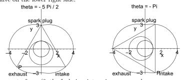
From  $\theta = -5\pi/2$  to  $\theta = -\pi$ , the fuel-air mixture is injected through the open intake valve on the lower right side:
