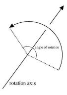
If the axis of rotation is oriented, we can say about *clockwise* or *counterclockwise* rotations (with respect to the view from the positive semi-axis).
