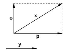
$\mathbf{p} = \text{orthogonal projection of } \mathbf{x} \text{ onto } \mathbf{y}$
