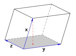
Parallelepiped is a prism. (Volume) = (area of the base)  $\times$  (height) Area of the base =  $|\mathbf{y} \times \mathbf{z}|$  Volume =  $|\mathbf{x} \cdot (\mathbf{y} \times \mathbf{z})|$
