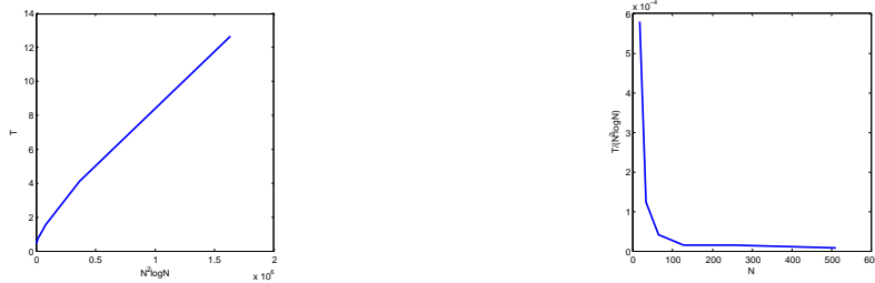
(a) Plot of CPU timings versus N^2 \log N where N^2 is the total number of points in the discretization of the domain. (b) Plot of T/(N^2 \log N) versus N where N^2 is the total number of points in the discretization of the domain.
