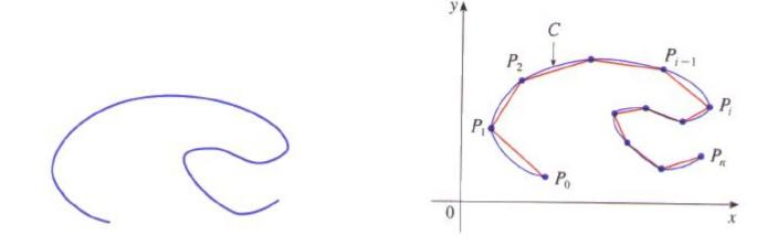
Then the length of the curve(arc length) is given by  $L = \lim_{n \to \infty} \sum_{i=1}^{n} |P_{i-1}P_i| = \lim_{n \to \infty} \sum_{i=1}^{n} \Delta s_i$
