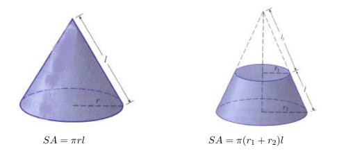
The surface area of a curve rotated about the x-axis:
