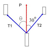
T1 and T2 are the vectors that represents the tensions on the cables from the tug boats. P is the resultant vector representing the path of the ship.
