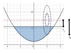
$$V = \int_{-3}^{3} \pi \left[ r_o^2 - r_i^2 \right] dx = \int_{-3}^{3} \pi \left[ (13 - x^2)^2 - 4^2 \right] dx = \int_{-3}^{3} \pi \left( 169 - 26x^2 + x^4 - 16 \right) dx$$
