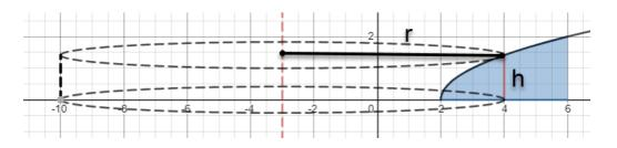
This is a dx integral since the slice (solid red line segment) is perpendicular to the x-axis. r = x - (-3) = x + 3 (right - left)
