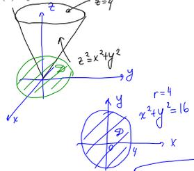
$$\begin{aligned} x^2 + y^2 &= r^2 \\ x &= r \cos \theta \\ y &= r \sin \theta \\ z &= z \end{aligned}$$
