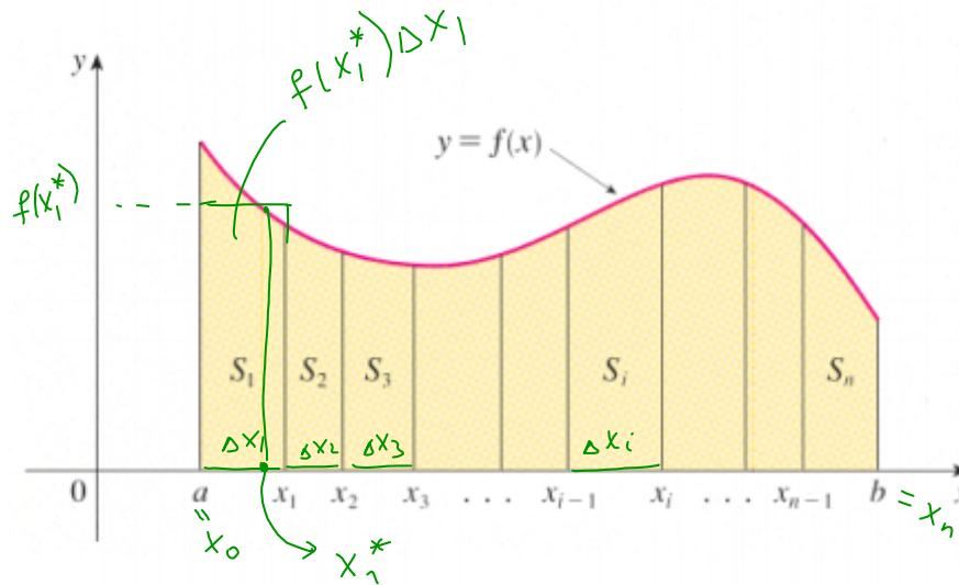
Approximate the strips  $S_1, S_2, \dots, S_n$  by rectangles  $R_1, R_2, \dots, R_n$ .
