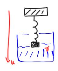
Damping force is proportional to instanteneous velocity
