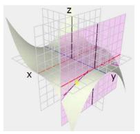
**Solution**: Since y is constant on this curve, it is the <u>x-Trace</u> and the slope of the tangent is the <u>x-Partial Derivative</u>.
