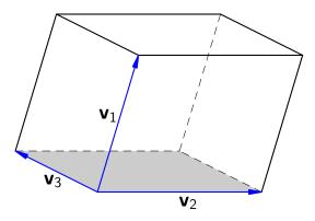
volume( $\Pi$ ) = |det B|, where  $B = (\mathbf{v}_1, \mathbf{v}_2, \mathbf{v}_3)$ . Note that the parallelepiped  $\Pi$  is the image under  $L_B$  of a unit cube whose adjacent edges are  $\mathbf{e}_1, \mathbf{e}_2, \mathbf{e}_3$ .
