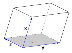
Parallelepiped is a prism. (Volume) = (area of the base) × (height) Area of the base =  $\|\mathbf{y} \times \mathbf{z}\|$ Volume =  $|\mathbf{x} \cdot (\mathbf{y} \times \mathbf{z})|$
