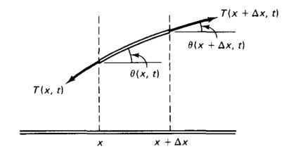
**perfectly flexible string:** no resistance to bending  $\theta(x, t)$  = angle between the horizon and the string
