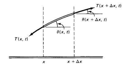
vertical component of tensile force =  $T(x + \Delta x, t) \cdot \sin \theta(x + \Delta x, t) - T(x, t) \cdot \sin \theta(x, t)$
